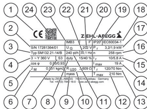
Example name plate ZAtop SM132
