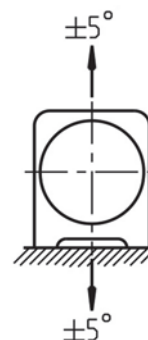
Resulting rope force ZAtop SM132.../BS without lateral form lock support
