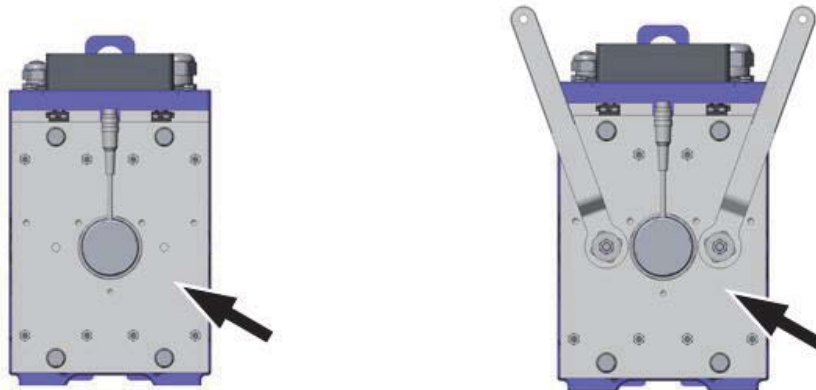
Brake with mechanical hand release system
